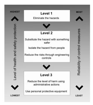
The ways of controlling risks can be ranked from the highest level of protection and reliability to the lowest, as shown in the adjacent diagram.
